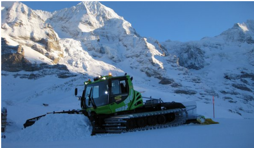
Pistenbully E+ with diesel-electric drive
