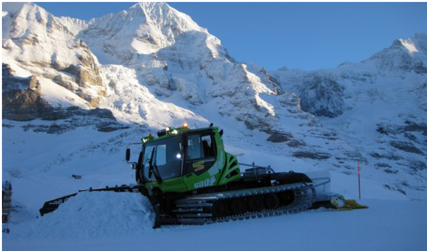
Pistenbully E+ with diesel-electric drive
